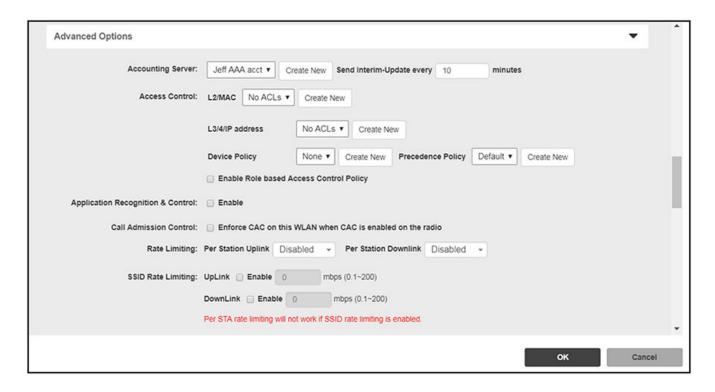
FIGURE 3 Configure Secure SSID on the SmartZone controller
