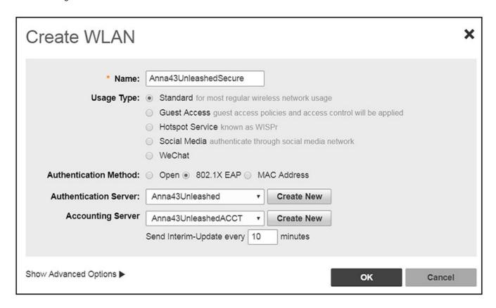
The SSIDs are now configured on the wireless LAN controller. When the user connects to the onboarding (open) SSID they are redirected to the Cloudpath web page. When the user successfully completes the enrollment process, they are migrated to the secure SSID.
