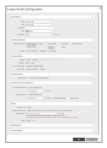
FIGURE 4 Configure Secure SSID on the Unleashed controller
